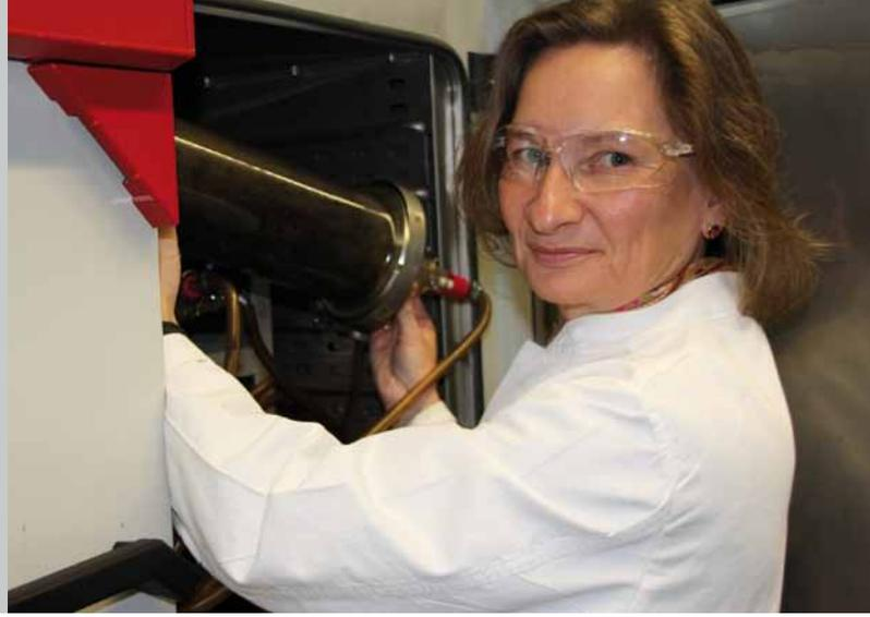
We inspect samples of the fermenter broth and then see how fast the substrates are converted into biogas within five days. We then know if it is optimal or if it has deficits.
